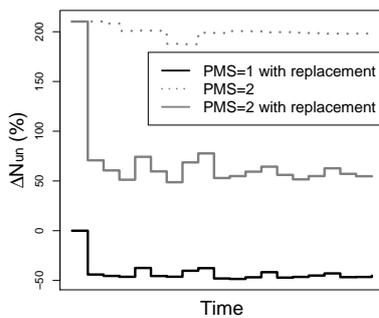
Figure 5: Mean number of system undesirable events for the three different maintenance strategies compared to the current one ( $N_{un}$  : number of undesirable events)
