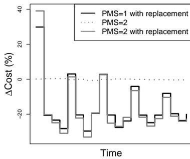
Figure 4: Mean system maintenance cost for the three maintenance strategies compared to the current one
